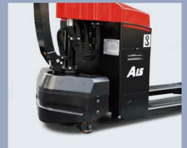
Auxiliary wheels are equipped to have better stability
